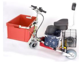
11.) Place the crate on the **support platform (A)** and align the center mark with the steering column. Place the straps around the **omega-shaped spacer (C)**, connect the clips and pull to tighten. Attach the two **bungees (H)** between the crate and the cane holders. The bungees reduce the possibility of lateral tilting.
