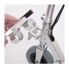
1.) Loosen the two mounting bolts, remove the footrest assembly and replace it with the adapter plate.
